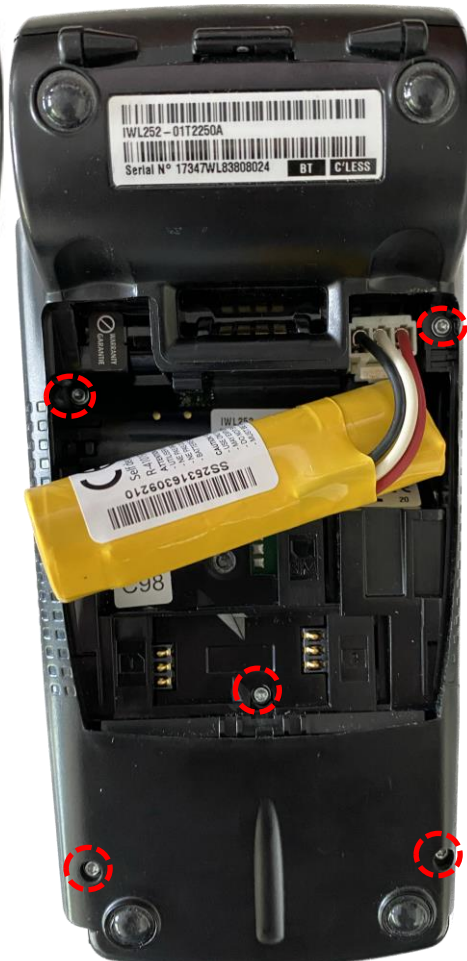
Rear View (Open) showing screws for inspection
